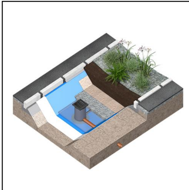
Figure 3 Hydroplanter Flex – flexible raingarden system (Source: GreenBlue Urban – [Ref. 10])
